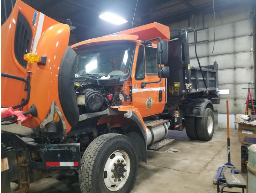
Figure 2 - Truck getting new turbocharger installed
